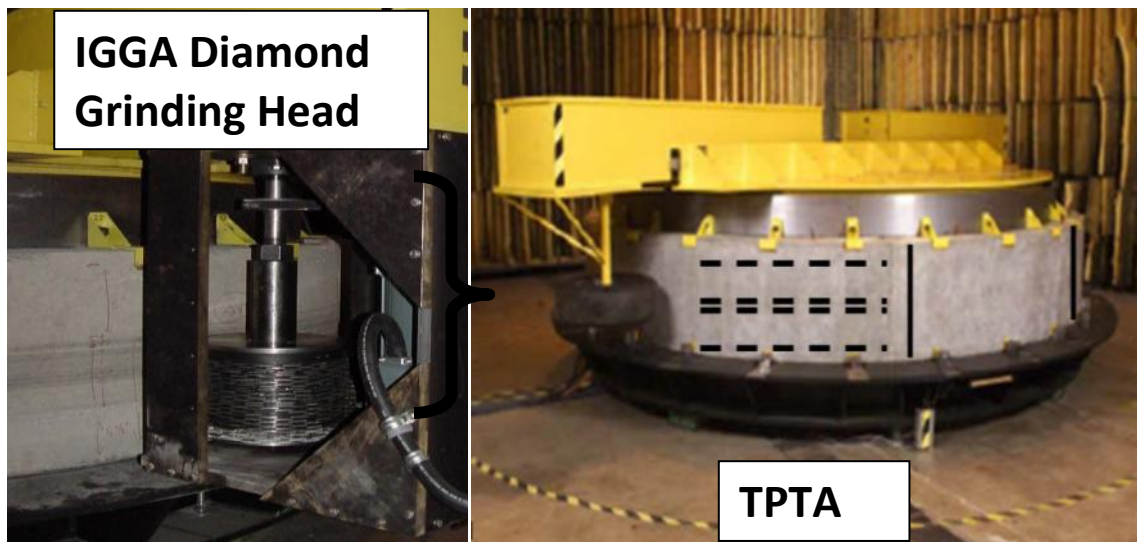
Figure 1- Purdue Tire Pavement Test Apparatus and IGGA Diamond Grinding Head 2
