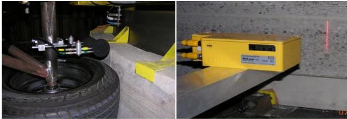
Figure 2- OBSI and RoLine™ Test Equipment Mounted to TPTA 2
