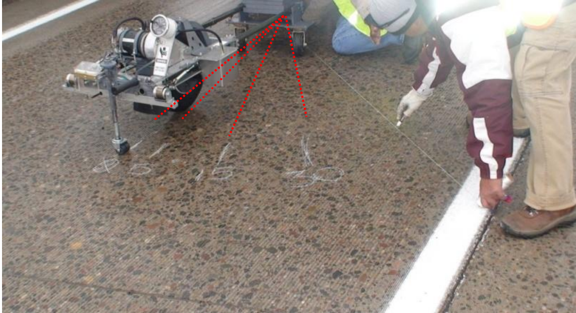
Figure 28 CT-342 Measuring Friction at Various Angles at MnROAD 17
