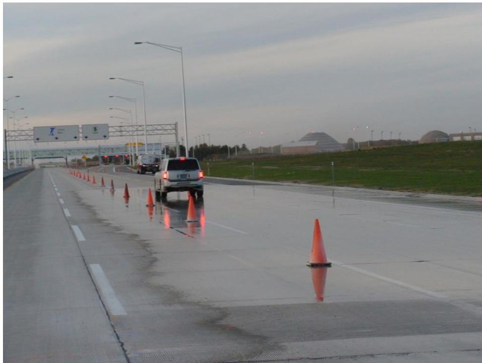
Figure 26 SUV Stopping Distance Testing on I-355
